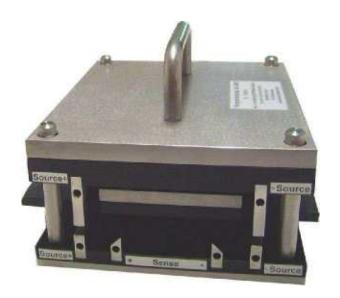
The four-pole electrode VE - D 991 was developed for the measuring of the volume resistivity of electrically conductive and antistatic materials according to the four-pole method.
