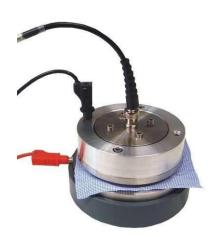
Surface measurement with grounded baseplate
