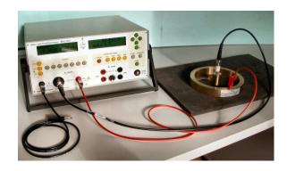
Measuring surface resistance with FGE 1 in connection with Milli-TO 3 (optional)
