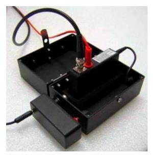
KB-HOW1 with HOW 1 (optional) and calibration resistor (optional)
