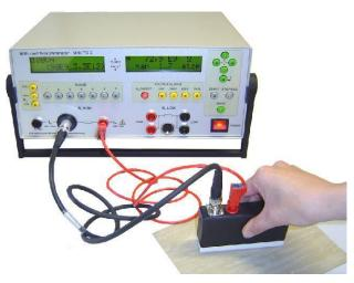
Hand-operated measuring HOW 1 with Milli-TO 3 (optional)
