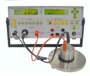
surface measurement with grounded baseplate GP 14 (optional) and Milli-TO 3 (optional)
