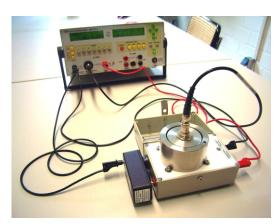
KB-FE50 with FE 50\*, calibration resistor\* and Milli-TO 3\* (\* optional)
