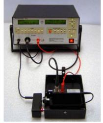
KB-HOW1 with HOW 1\*, calibration resistor\* and Milli-TO 3\* (\* optional)
