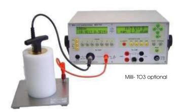
The powder electrode PE01 for the measuring of high-ohm volume resistances at pulverized specimen.
