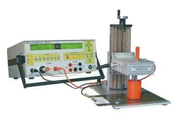
EH15/20 are suitable for the measurement of volume and surface resistance atsmall pads.
