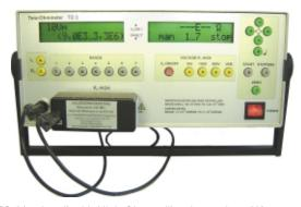
TO 3(optional) with High Ohm calibration resistor N8
