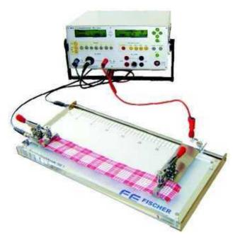
The textile strip electrode TSE 1 is suitable for measuring the electrical resistance of strips of textile fabrics which include improving the conductivity of electrostatic charges admixtures of materials whose resistance is much lower than that of the textile material.
