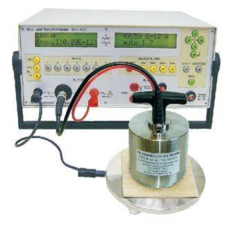
surface measurement with AE 30-DIN and grounded base plate GP 14 (optional) connected to Milli-TO 3
