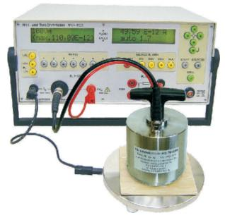
surface measurement with AE 30 and grounded base plate GP 14 (optional) connected to Milli-TO 3
