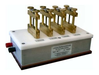
The four-pole bar electrode BPT 1 was developed for the measuring of the electric insulating resistance of solid insulate materials according to the standard DIN EN 62631-3-3:2016.
