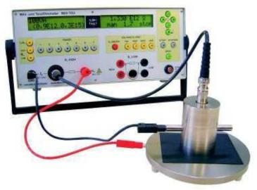
The protective ring electrode 3604FE is suitable for versatile measuring of volume resistance at small plate-shaped specimen.
