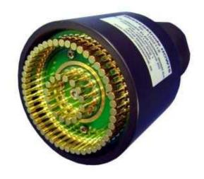
The HOW16 is a electrode arrangement to measure the resistance of surface layer according to EN, DIN und IEC.
