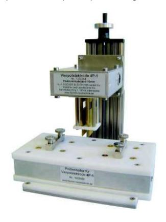
The four-pole electrode was developed for the measuring of the electric volume and surface impedance of conductive materials according to the four-pole method. The structure of the electrode complies with the norm DIN EN ISO 3915.
