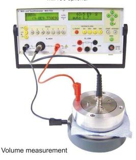
ring electrode in high-grade steel and aluminium quality
