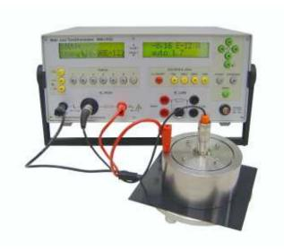
surface measurement with grounded baseplate GP 14 (optional) and Milli-TO 3 (optional)
