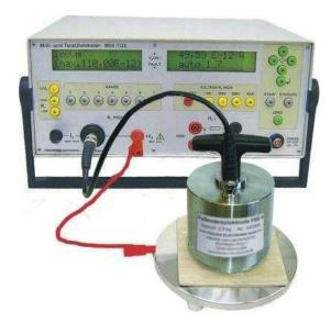
Volume resistance measurement with FBE 4 and earth plate GP 14 \* and Milli-TO 3 3
